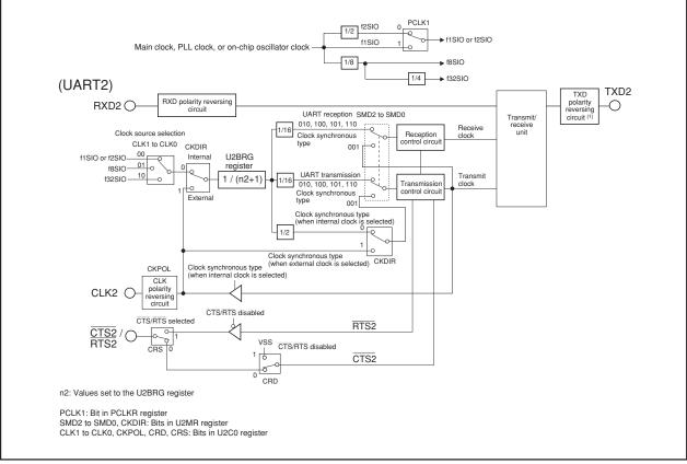
Figure 14.3 UART2 Block Diagram
